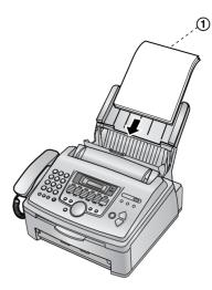
5 Attach the paper tray cover (①), then push back the tension plate (②).
